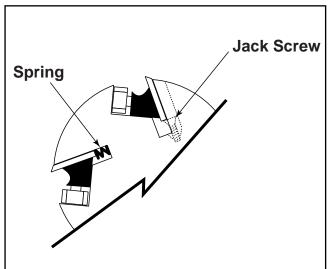
**Figure 13.** Typical placement of jack screws or springs.
